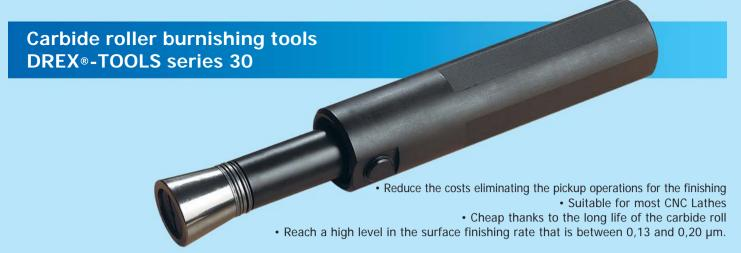
It is possible to burnish inside and outside diameters, fitting's radius or borders, shoulders and bar's end with only a single tool. **The carbide roller burnishing tools have been studied for being used on CNC lathes**. The surfaces to be burnish are prepared of turning with a roughness of 2-2,5 µm. The tool, put in the due working position, has used with a speed same of the turning's speed, obtaining a roughness of 0,13-0,20 µm. This replace the need of a pickup operation.
