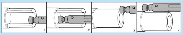
**D30-30-0** It is the right tool for small size parts; with its roll diameter 30,2 and an overall length of 241 mm it is possible to burnish holes beginning from a diameter 35 mm and for a depth of 75 mm.
