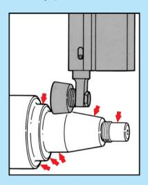
It is possible to change your turning CNC centre in a finishing centre with the Drex®-Tools carbide O.D. roller burnishing tool.
